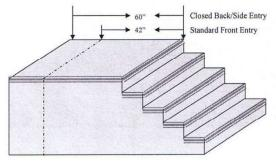
DO NOT USE SALT or DEICER ON PRECAST STEPS! Side-Entry Steps only available in 4' wide. Short or no platform steps also available via special order. Railings for all sizes except special orders in stock. Concrete strength fc 4000PSI@28 days. Density 150 PCF. Cement, Portland Type II or III, ASTM C150-81 Admixtures, air & plasticizers per ASTM C233-82
